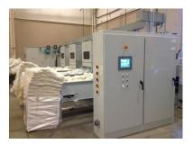
The CCS *MaxLoft* weight control system is a PLC based touch screen system that is manufactured with UL/CE compliant off the shelf components such as Siemens, Allen-Bradley and others. The *MaxLoft* system includes recipe management, active weigh control, trending, reporting, help screens, remote support and multilingual text.
