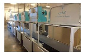
CCS *MaxLoft* high speed openers are manufactured in many different styles; the standard openers are horizontally or vertically fed. The openers can be configured with metallic wire wound cylinders, fully lagged cylinders and claw tooth cylinders depending on the application. CCS *MaxLoft* Blending and Opening systems are capable of producing as much as 1,500 to 2,500 kilos per hour depending on the fiber type, denier, staple length and blend percentages.
